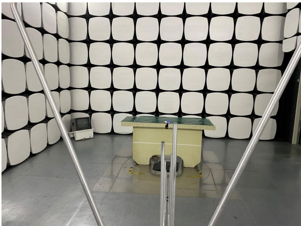
**Radiated Emissions Test Photos****Above 1 GHz**
