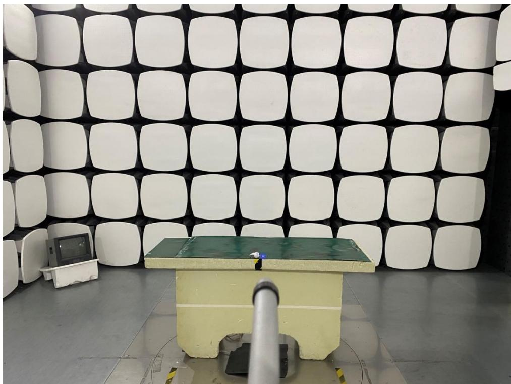
**Radiated Emissions Test Photos****30 MHz to 1 GHz**
