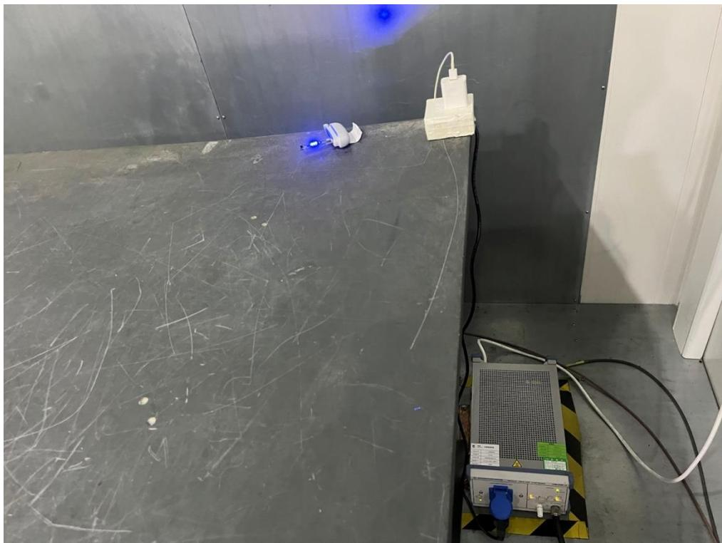
**Radiated Emissions Test Photos****9 kHz to 30 MHz**
