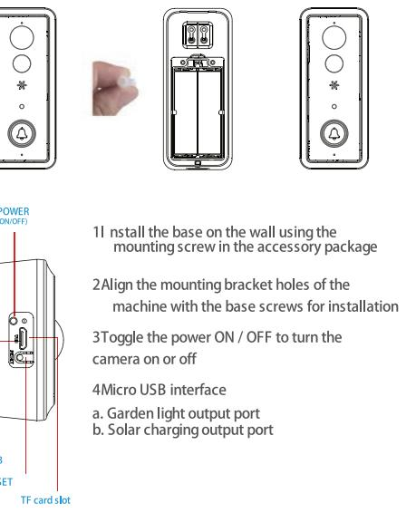
5Press the reset button for 5 seconds, waiting for the indicator light turn to red slow flash
