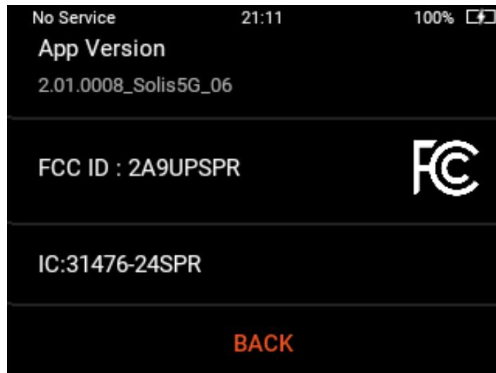
Above regulatory information is secured and implemented in a factory-set-unalterable format. End user can easily to access regulatory information without SIM card.
