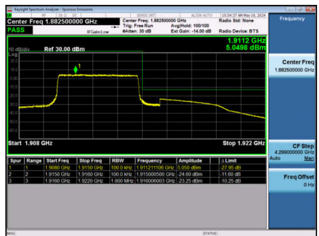
LTE Band 25-5MHz-QPSK-HCH-25RB#0
