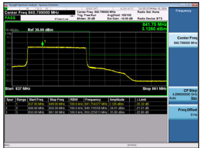
LTE Band 26_P22-15MHz-QPSK-LCH-75RB#0
