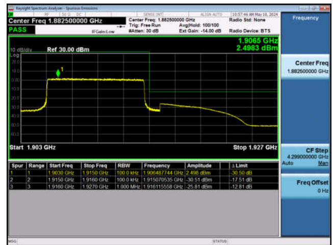
LTE Band 25-15MHz-QPSK-LCH-75RB#0
