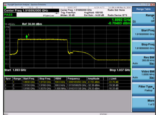
LTE Band 25-20MHz-QPSK-HCH-100RB#0
