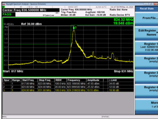
LTE Band 26_P22-5MHz-QPSK-HCH-1RB#24
