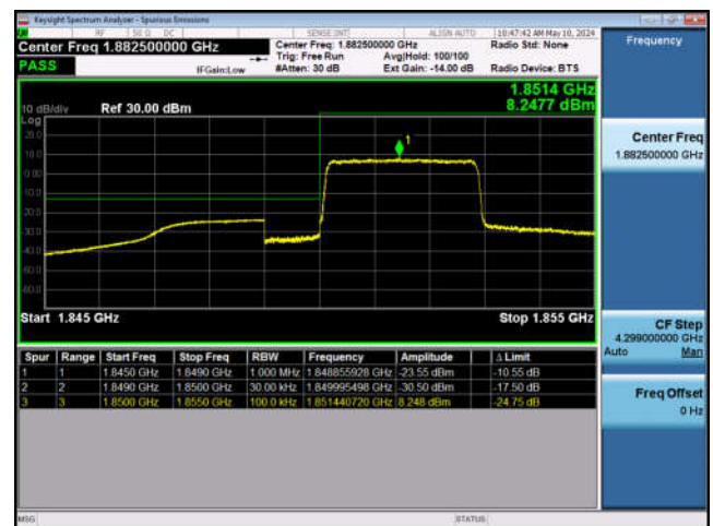
LTE Band 25-3MHz-QPSK-LCH-15RB#0
