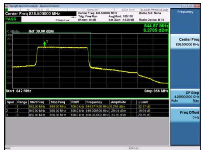
LTE Band 26_P22-5MHz-QPSK-HCH-25RB#0
