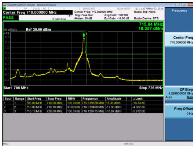
LTE Band 17-10MHz-QPSK-LCH-1RB#0
