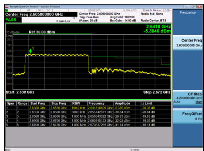
LTE Band 41-15MHz-QPSK-HCH-75RB#0
