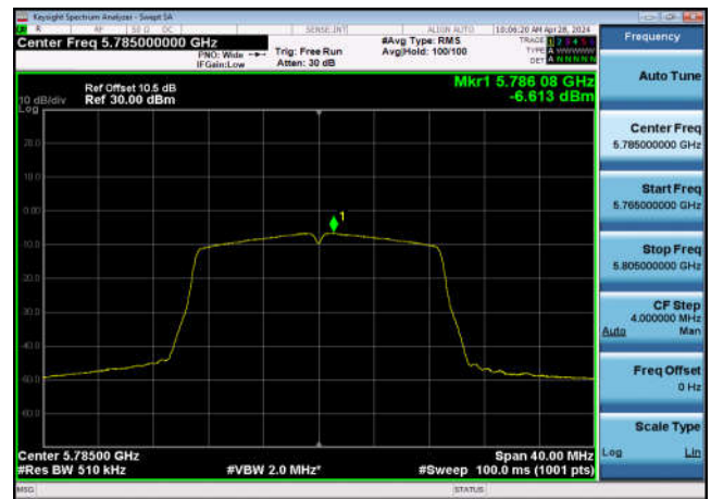
U-NII-3 Power spectral density-802.11 n(40MHz),5755MHz,Ant1
