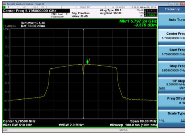
U-NII-3 Power spectral density-802.11 a(20MHz),5785MHz,Ant1
