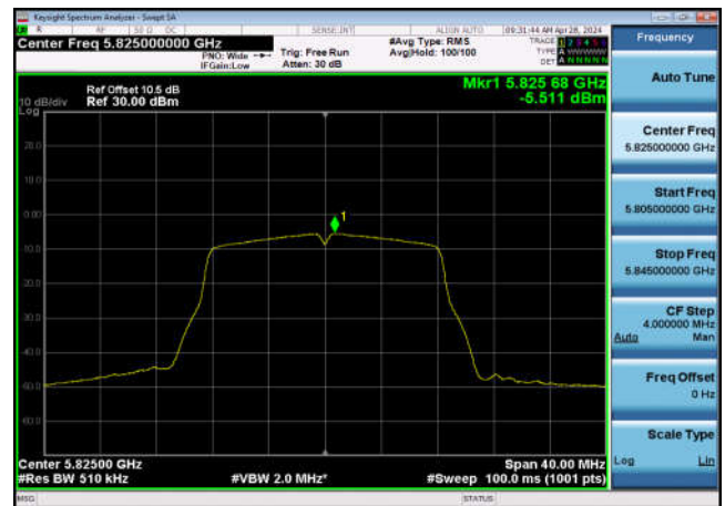
U-NII-3 Power spectral density-802.11 ac(20MHz),5785MHz,Ant1
