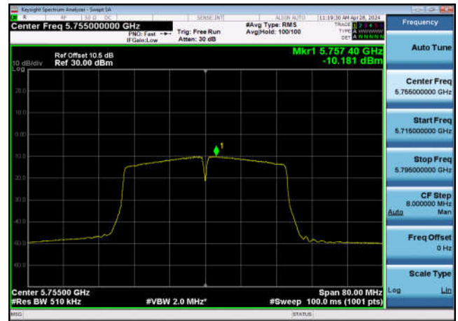
U-NII-3 Power spectral density-802.11 ac(80MHz),5775MHz,Ant1
