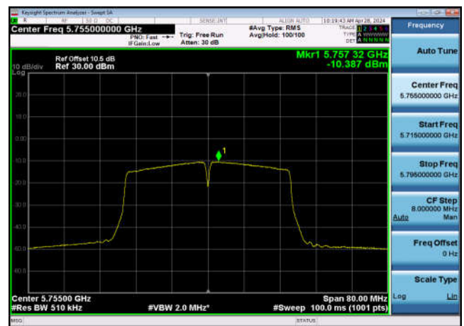
U-NII-3 Power spectral density-802.11 n(40MHz),5755MHz,Ant1
