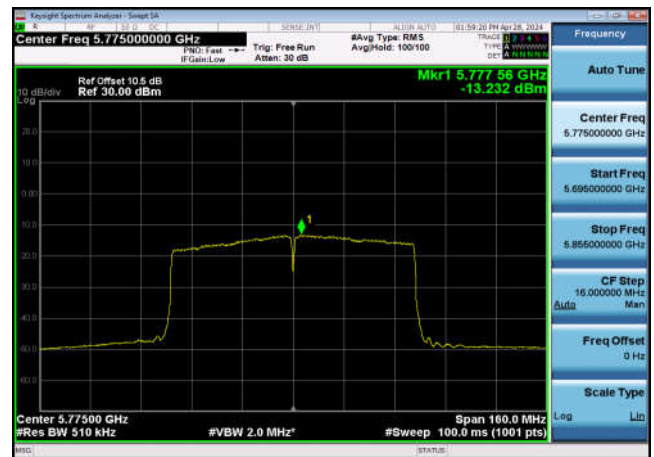
U-NII-3 Power spectral density-802.11 ac(80MHz),5775MHz,Ant1
