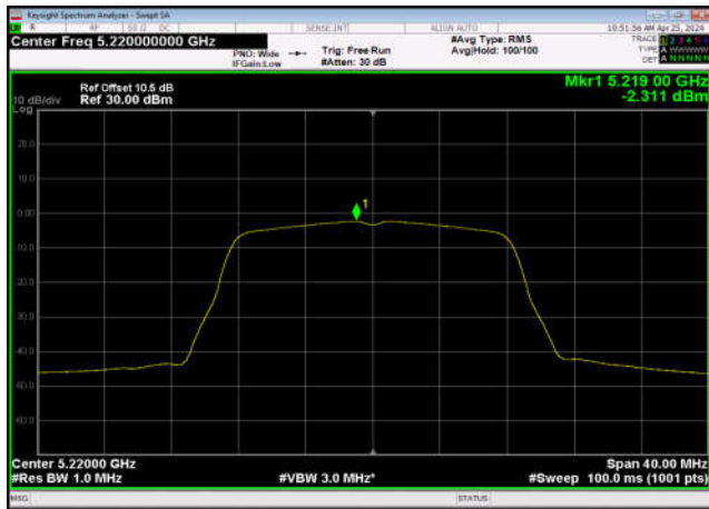
U-NII-1 Power spectral density-802.11 ac(20MHz),5180MHz,Ant1
