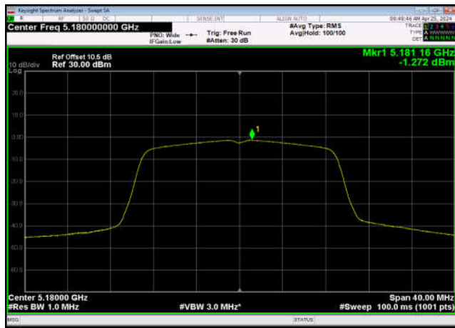
U-NII-1 Power spectral density-802.11 n(20MHz),5240MHz,Ant1
