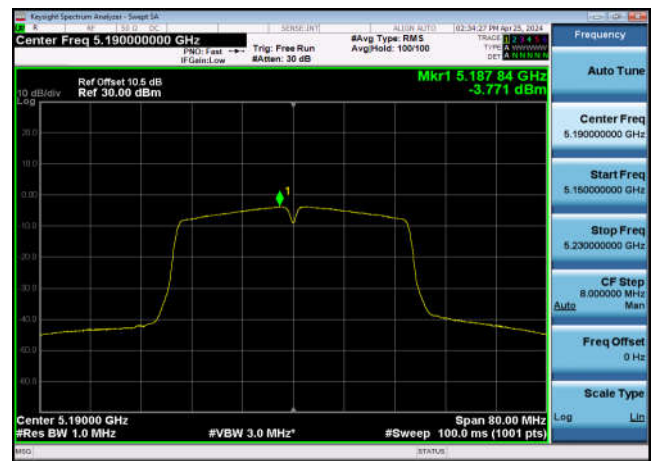
U-NII-1 Power spectral density-802.11 a(20MHz),5180MHz,Ant1
