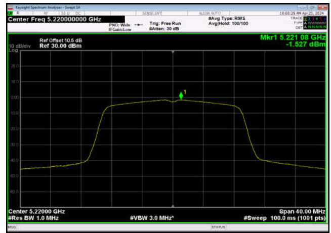
U-NII-1 Power spectral density-802.11 n(40MHz),5190MHz,Ant1
