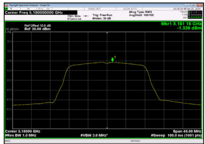
U-NII-1 Power spectral density-802.11 a(20MHz),5180MHz,Ant1
