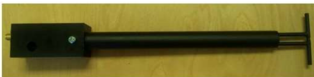
Figure 1 – MVG COMOSAR Validation Dipole
