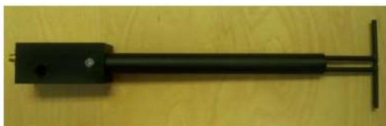
Figure 1 – MVG COMOSAR Validation Dipole
