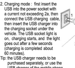
2. Charging mode: first insert the USB into the power socket with a current not exceeding 2a, then connect the USB charging cable, then insert the USB charger into the charging socket under the vehicle. The USB socket light is on, indicating that charging starts, and the light goes out after a few seconds (charging is completed about 60 minutes). Tip: the USB charger needs to be purchased separately, or use the USB charger of the mobile phone.
