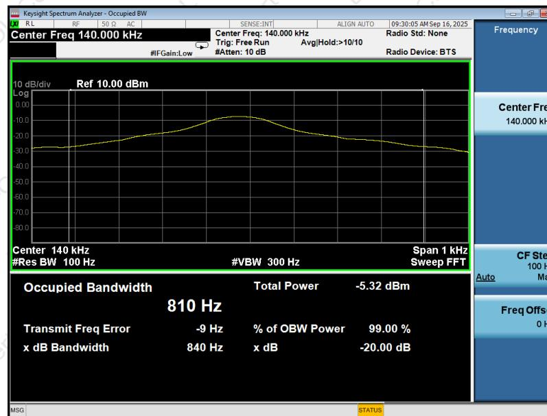
Note: The measured signal is Cw-like, adjusting the RBW per C63.10 would not be practical since measurement bandwidth will always follow the RBW. The RBW is set to 300 Hz to perform the occupied bandwidth test.
