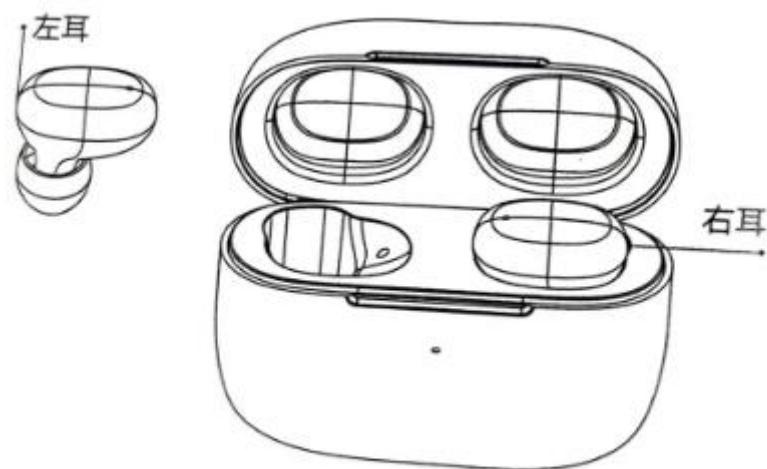
Choose a suitable size from the three earplugs of different sizes provided, and assemble it on the sound outlet of the hearing aid.
