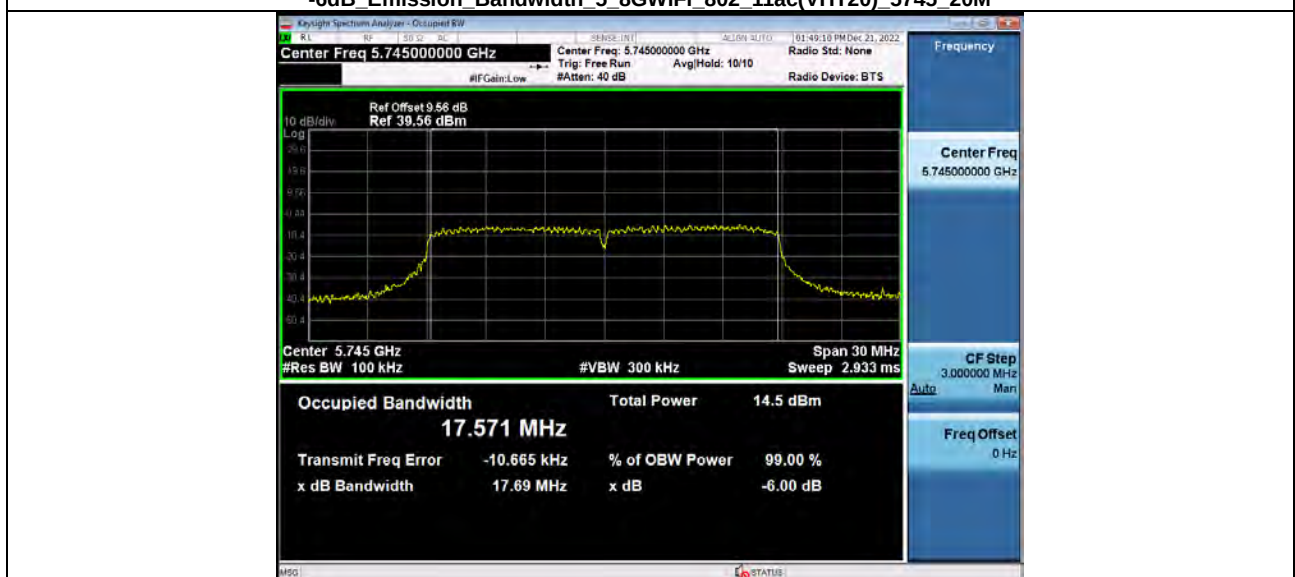
-6dB Emission Bandwidth 5_8WiFi 802_11ac(VHT20) 5785_20M
