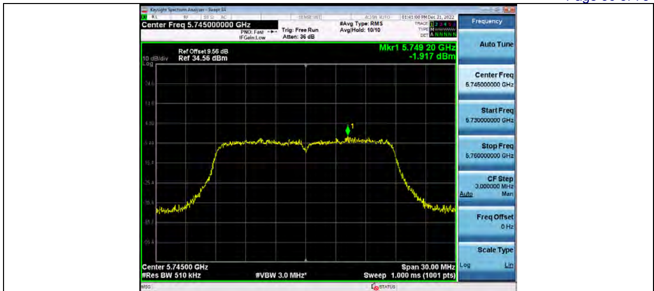
Power Spectral Density 5_8WiFi 802_11n(HT20) 5785_20M
