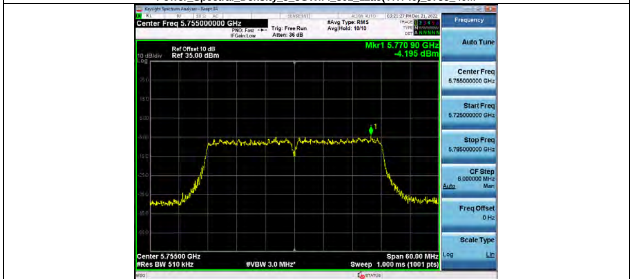
Power_Spectral_Density 5_8WiFi 802_11ac(VHT40)_5755_40M
