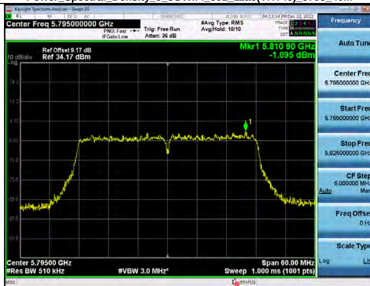
Power_Spectral_Density 5_8WiFi 802_11ac(VHT40) 5795_40M
