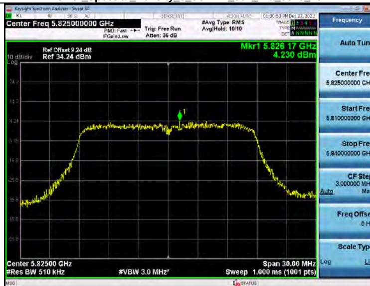
Power Spectral Density 5_8WiFi 802_11a 5825_20M
