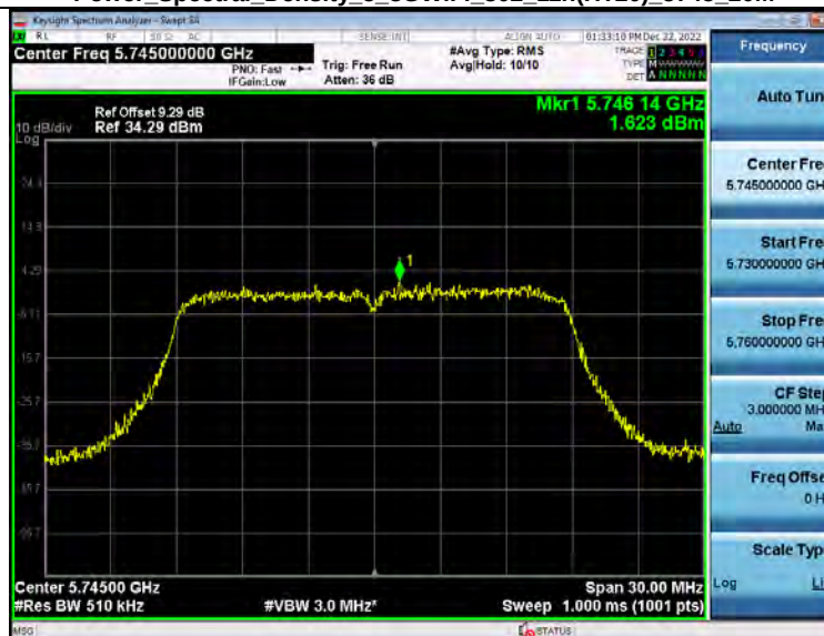
Power Spectral Density 5_8WiFi 802_11n(HT20) 5745_20M
