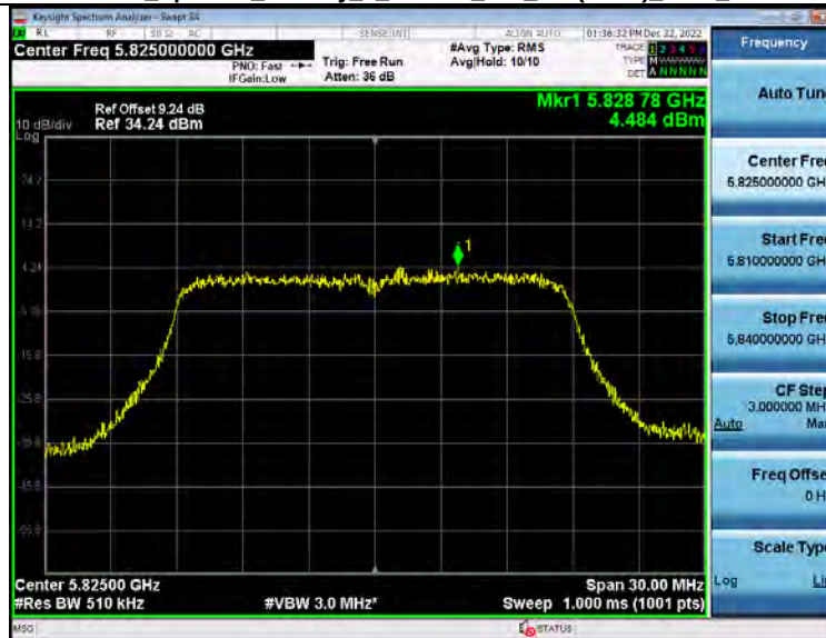
Power Spectral Density 5_8WiFi 802_11n(HT20) 5825_20M
