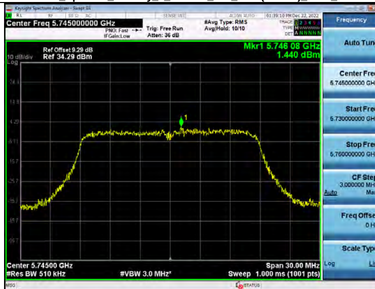
Power Spectral Density 5_8WiFi 802_11ac(VHT20) 5745_20M
