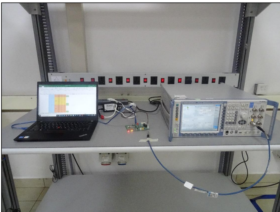
Conducted emission test setup
