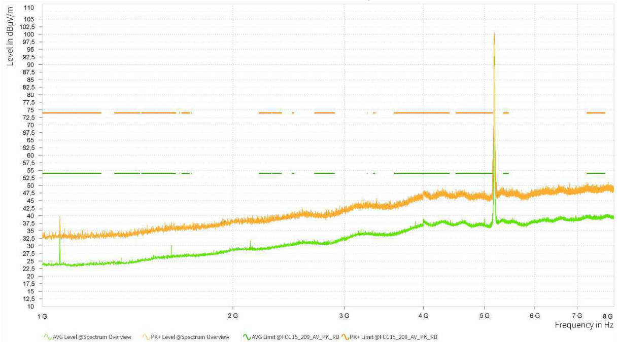
Plot 305: RSE 1 GHz – 8 GHz, Mode 1, CH36, horizontal / vertical polarisation
