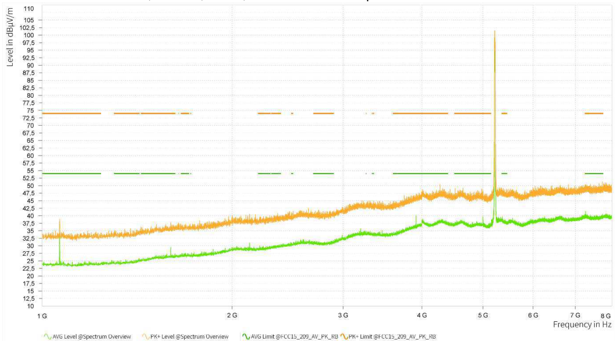
Plot 306: RSE 1 GHz – 8 GHz, Mode 1, CH44, horizontal / vertical polarisation
