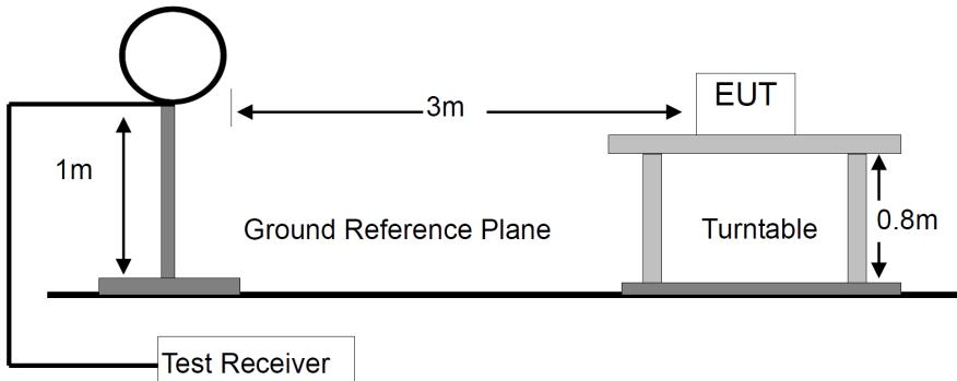
For Radiated Emission 30-1000MHz
