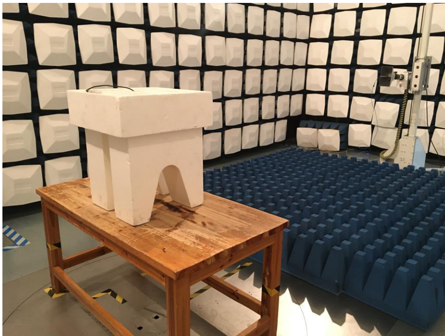
Test Setup For Radiated Emission (Above 1GHz)
