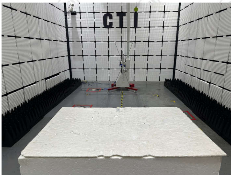
Radiated emission Test Setup-2 (30MHz~1GHz)
