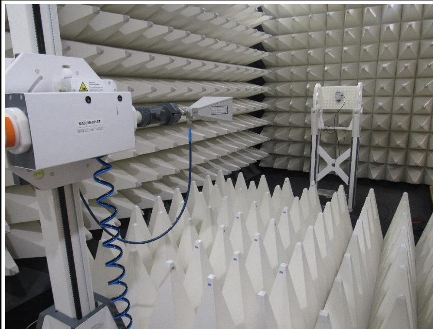
Setup for measurements above 1 GHz
