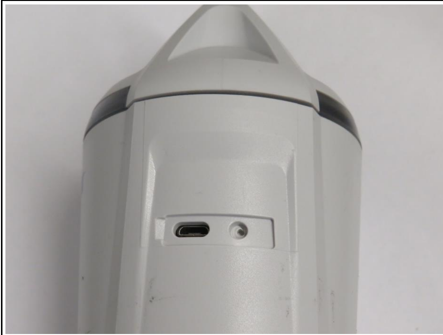
12 EUT USB-connector open (only for documentation)
