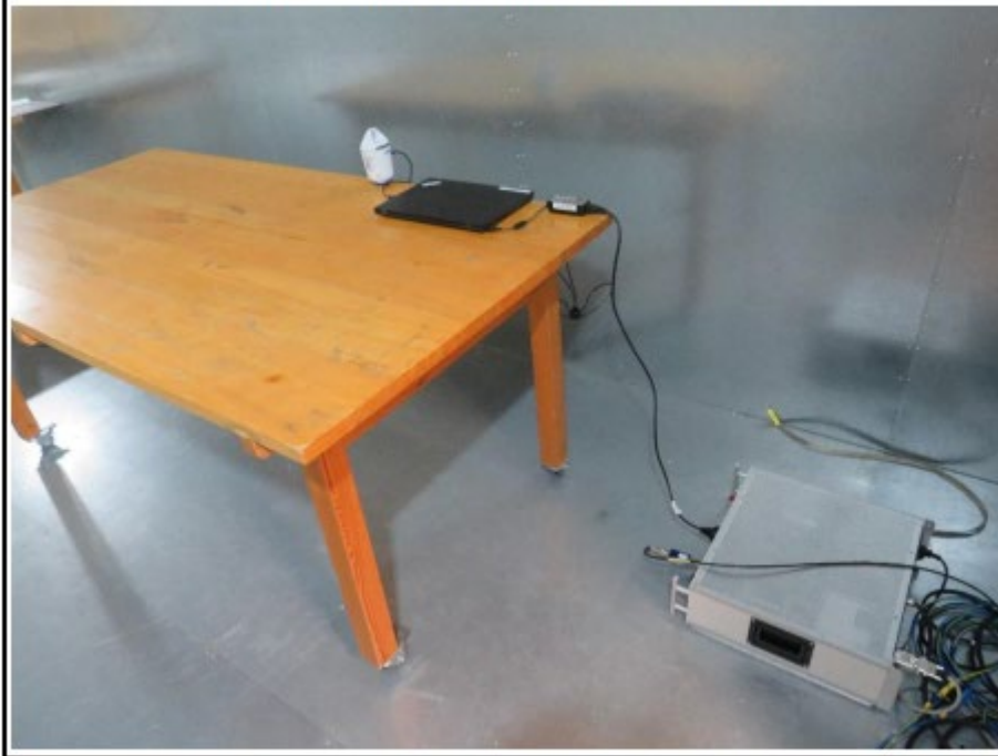
Setup for measurement 150 kHz - 30 MHz
