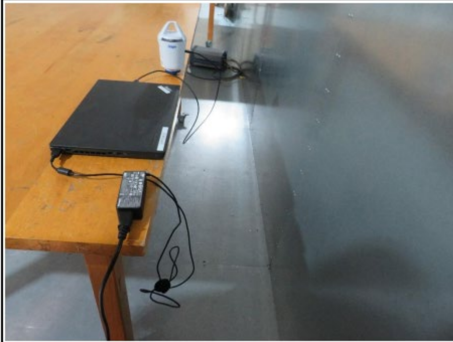
Setup for measurement 150 kHz - 30 MHz
