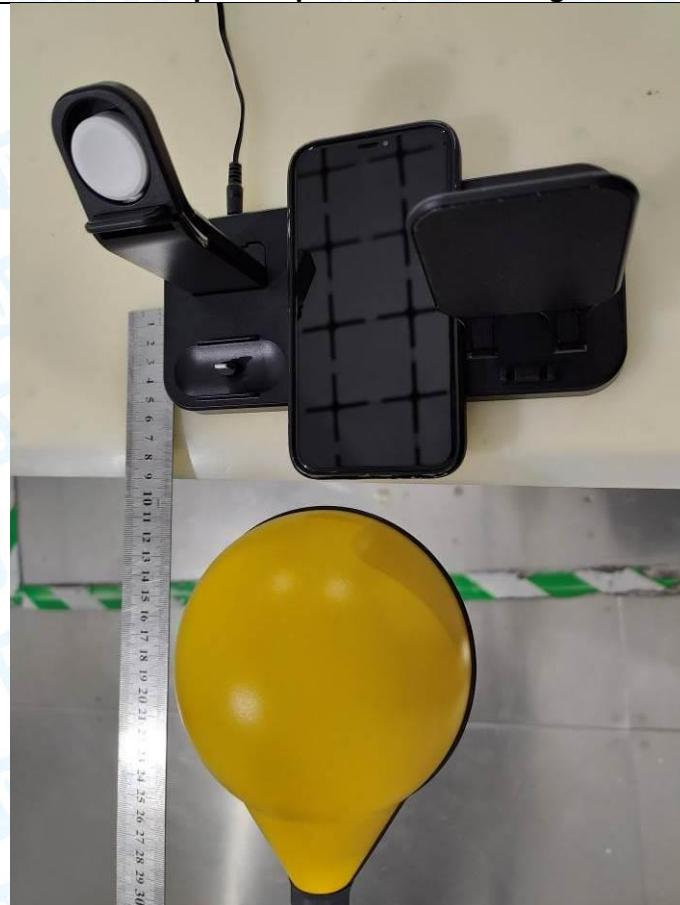
**H-Field Strength-15cm****Test Position D - Exposure photo from side edge surface-Right**
