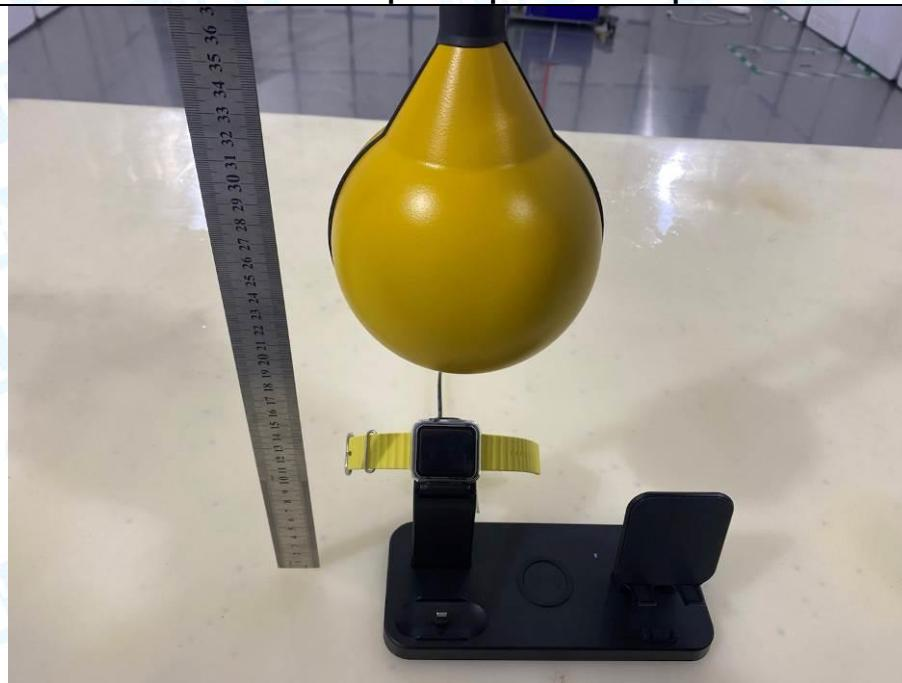
**H-Field Strength-15cm (Phone Ant2)****Test Position E - Exposure photo from top surface**
