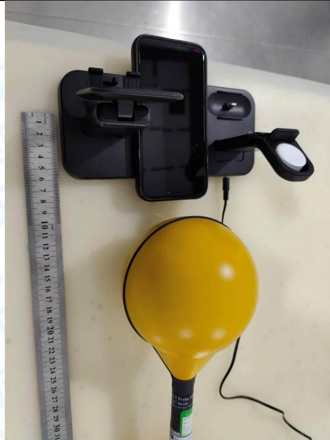
**H-Field Strength-15cm****Test Position B - Exposure photo from side edge surface-Left**
