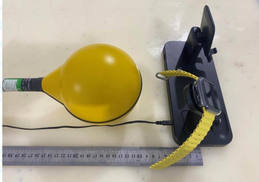
**H-Field Strength-15cm****Test Position B - Exposure photo from side edge surface-Left**
