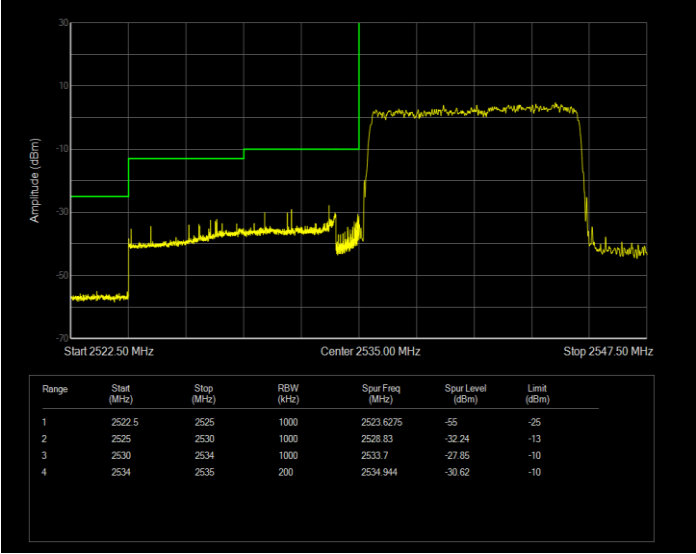
Band41(2535-2655) QAM16 BW=10MHz Channel=40090 RB Size=50 Position=#0
