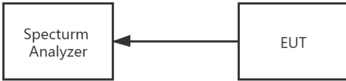
The EUT is connected to the Spectrum Analyzer; the RF load attached to the EUT antenna terminal is 50Ohm; the path loss as the factor is calibrated to correct the reading. Tune the measurement with the spectrum analyzer's resolution bandwidth (RBW) = 100 kHz. In order to make an accurate measurement, the span is set to be greater than RBW.
