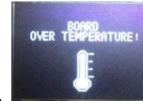
Indicates overheat and the motor will stop working.
