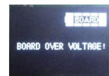
detects the battery voltage is too high. If the user continues to go downhill, the board will brake automatically to prevent user from doing that. This method can only protect the battery to a limited extent and cannot 100% guarantee for the battery safety.
