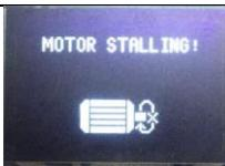
the screen of remote control indicates lock-up. If that happens, the user should stop running skateboard and check whether there is foreign matter struck in it, clear the foreign matter and run it again.
