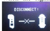
If the skateboard is accelerating, first the acceleration will stop slowly, then brake slowly automatically. If the skateboard is not accelerating, it will brake slowly. If the signal is lost, the remote control will search the device of skateboard, if it succeeds in searching and reconnecting, the remote control will short vibrate, the brake will be cancelled and return to normal operation.
