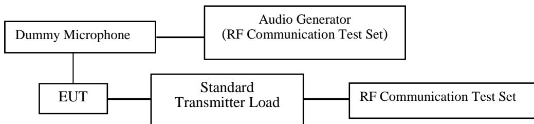
Setup Block Diagram for Audio Frequency filter:
