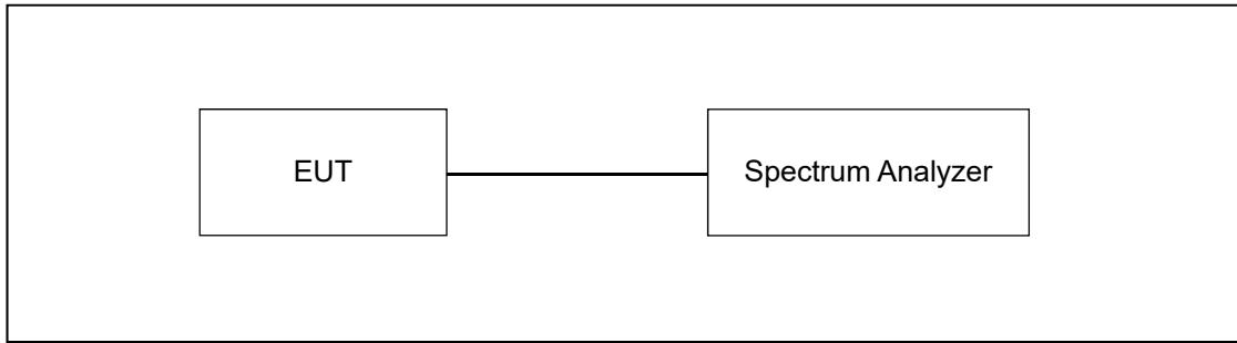
Using system management software, make a channel availability request to the database. Using the spectrum analyzer, confirm that the WSD operates at no more than the maximum power level indicated by the database and that the power level cannot be set to a higher level than indicated by the database at that specific location. If the device cannot reduce power, it must cease operation. Testing in accordance with KDB 416721 D01, III (2)(o).
