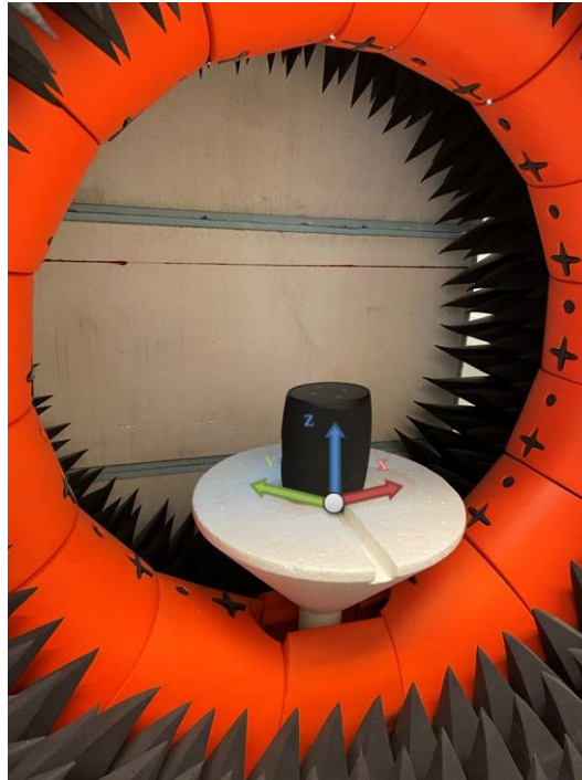
Figure 1: Test setup used for the antenna radiation pattern measurements
