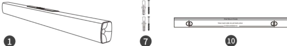
**Step2:** Using below part ⑩ as a size reference, punch holes on the wall.
