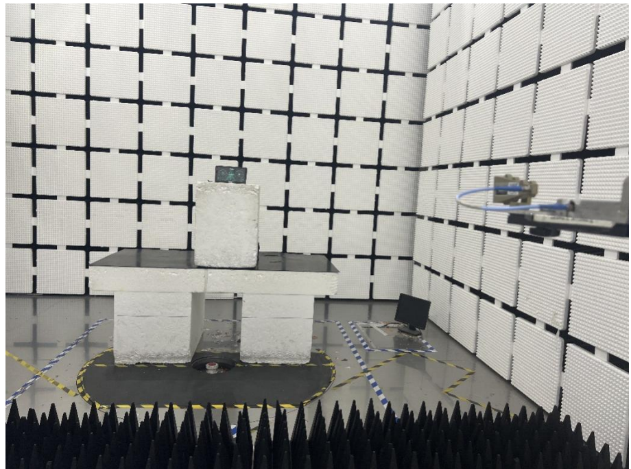
Radiation Emission Test Setup (Above 18GHz)
