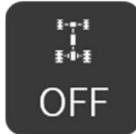
4WD icon shows the current mode of the vehicle. If 4WD icon is “ON”, the vehicle will operate in 4-Wheel Drive mode.
