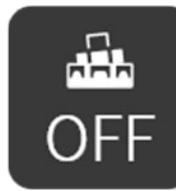
Horizontal mode icon shows the current mode of the vehicle. If Horizontal mode icon is “ON”, the vehicle will operate in Horizontal mode. When the engine is off, “OFF” is shown.
