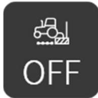
Draft mode icon shows the current mode of the vehicle. If Draft mode icon is “ON”, the vehicle will operate in Draft mode. When the engine is off, “OFF” is shown.
