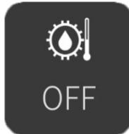
Transmission oil temperature icon shows the current temperature of the transmission oil. When the engine is off, OFF is shown instead of numbers.
