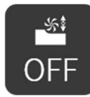
Depth mode icon shows the current mode of the vehicle. If Depth mode icon is “ON”, the vehicle will operate in Depth mode. When the engine is off, “OFF” is shown.
