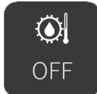
Transmission oil temperature icon shows the current temperature of the transmission oil. OFF is shown when the engine is off instead of numbers.
