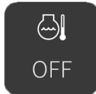
Coolant temperature icon shows current temperature of coolant. OFF is shown when the engine is off instead of numbers.
