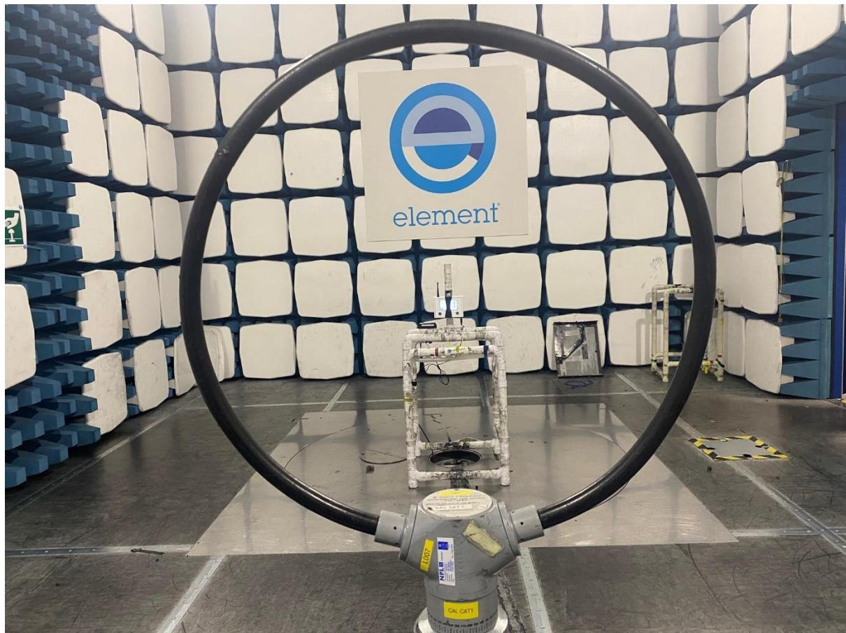
30MHz-1GHz Radiated tests
