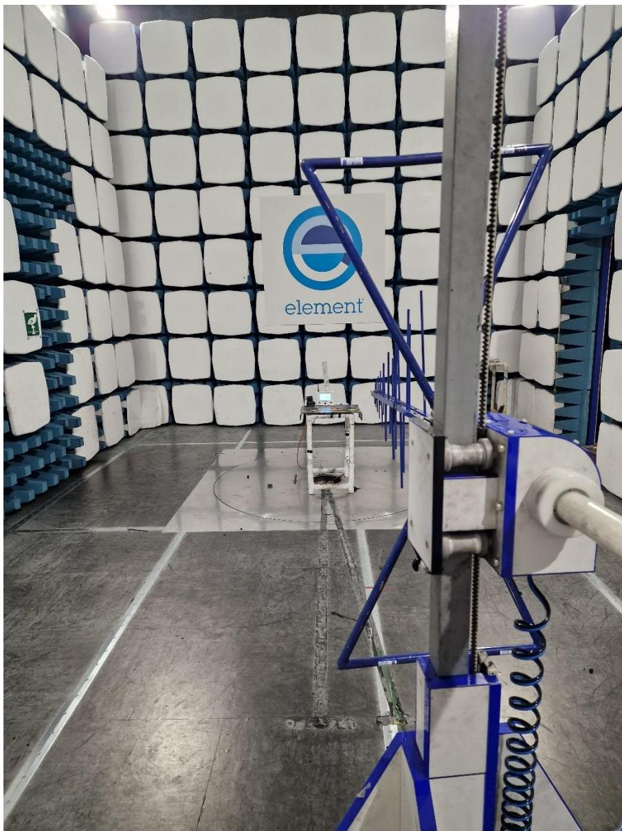
1GHz-10GHz Radiated tests
