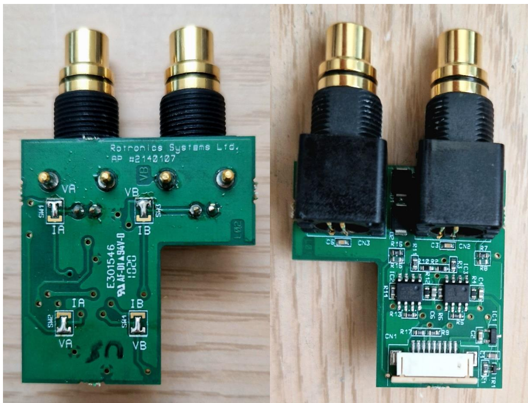
GENII/INST/200 0-10V Sensor interface PCBA
