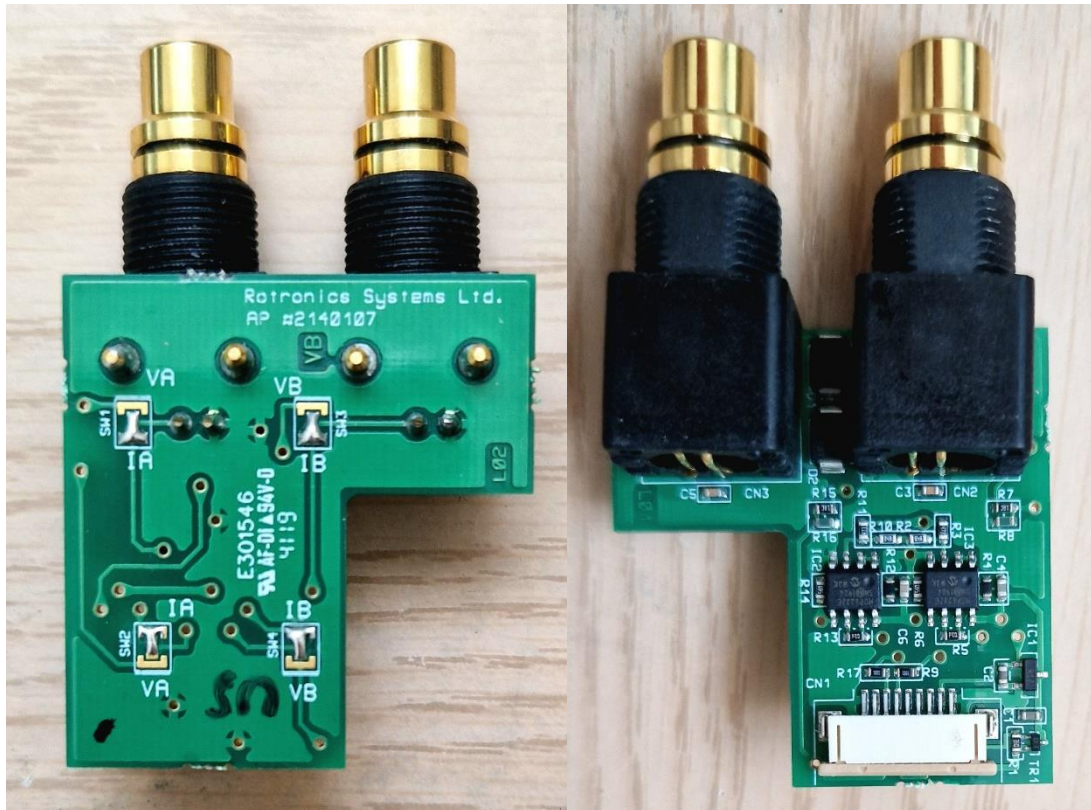
GENII/INST/200/A 4-20mA Sensor interface PCBA
