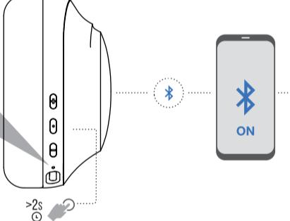
Press and hold the **middle button** for 2 seconds to power on and automatically enter pairing mode.
