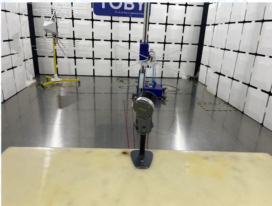
Photo of Setup for Radiated Emission (30MHz~1GHz)
