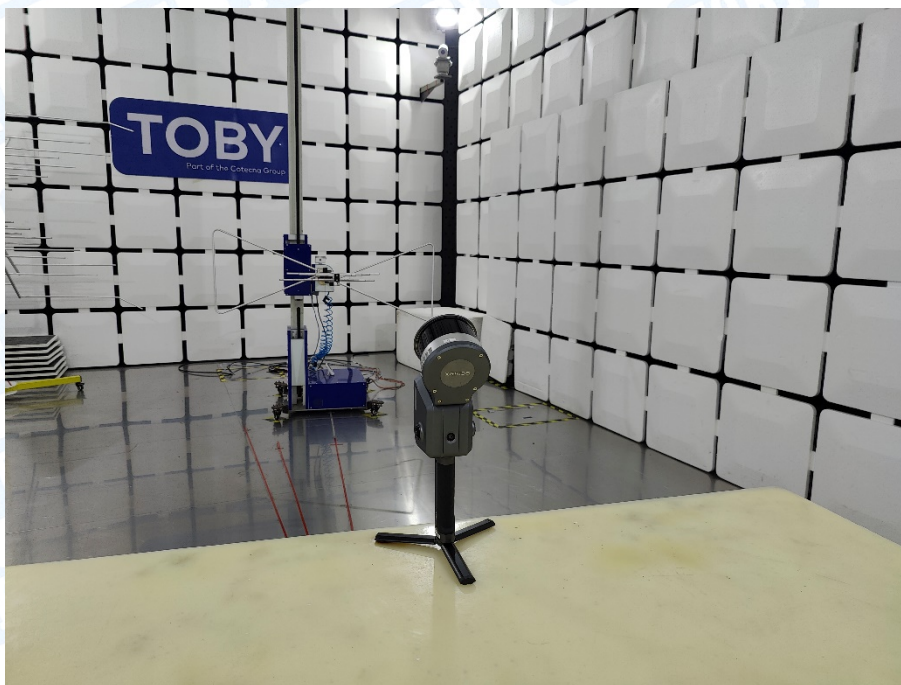
Photo of Setup for Radiated Emission (30MHz~1GHz)
