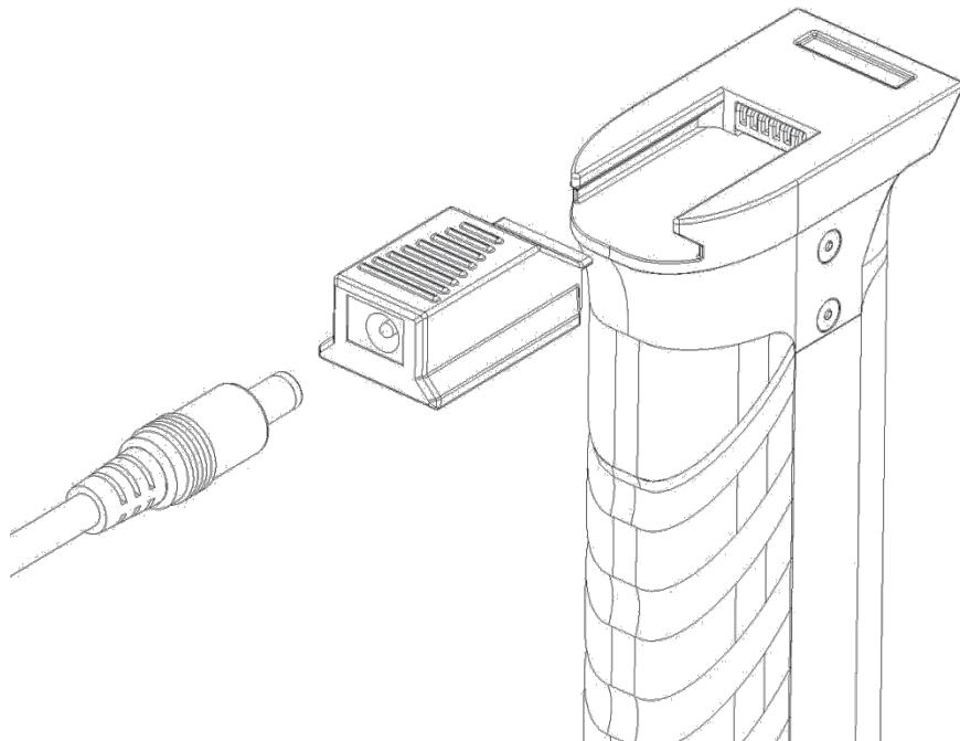
Use the standard charging cable and connect the charging adapter to the battery to charge the battery.
