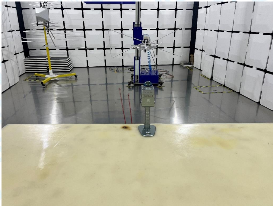
Photo of Setup for Radiated Emission (30MHz~1GHz)
