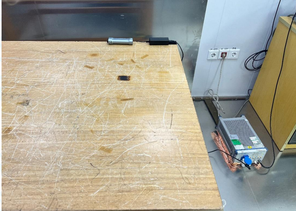
Photo of Setup for Radiated Emission (30MHz~1GHz)
