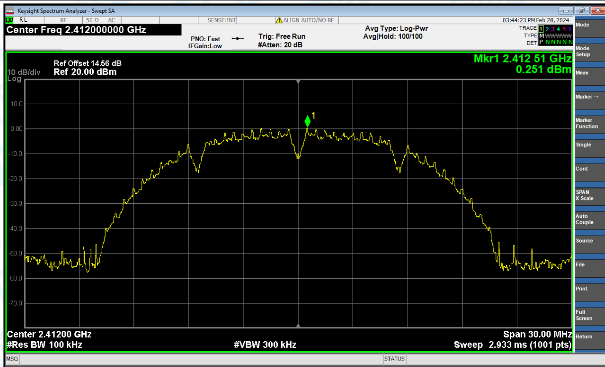
Tx. Spurious NVNT b 2412MHz Ant1 Emission
