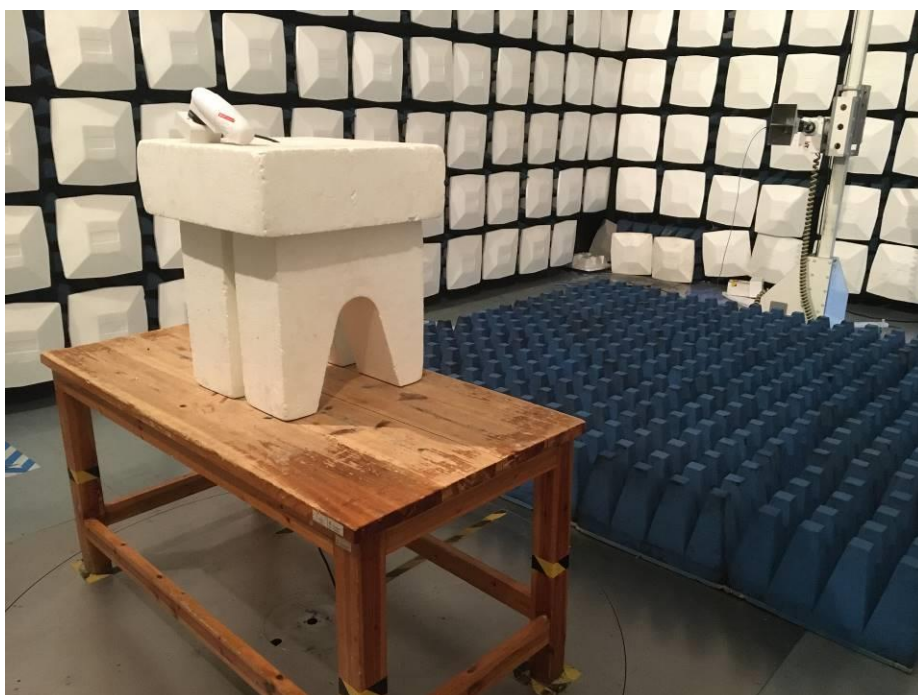
Test Setup For Radiated Emission (Above 1GHz)
