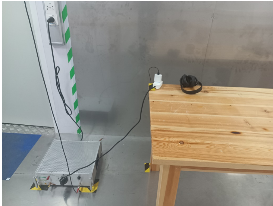
FCC: 2A9P5-A6 Photo of Conducted Emission Measurement
