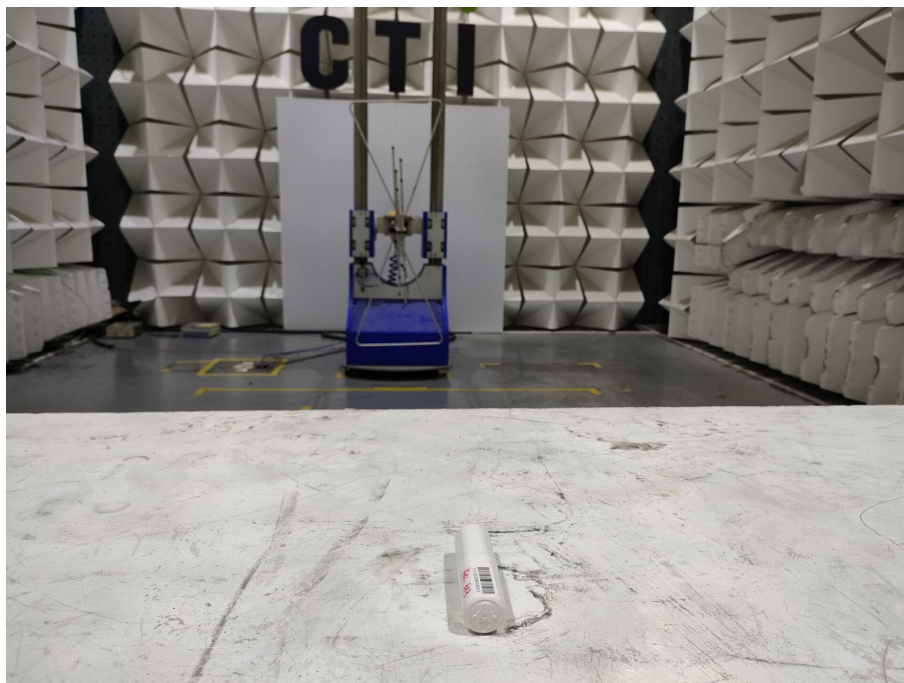
Radiated spurious emission Test Setup-2(Below 1GHz) (small) Close up
