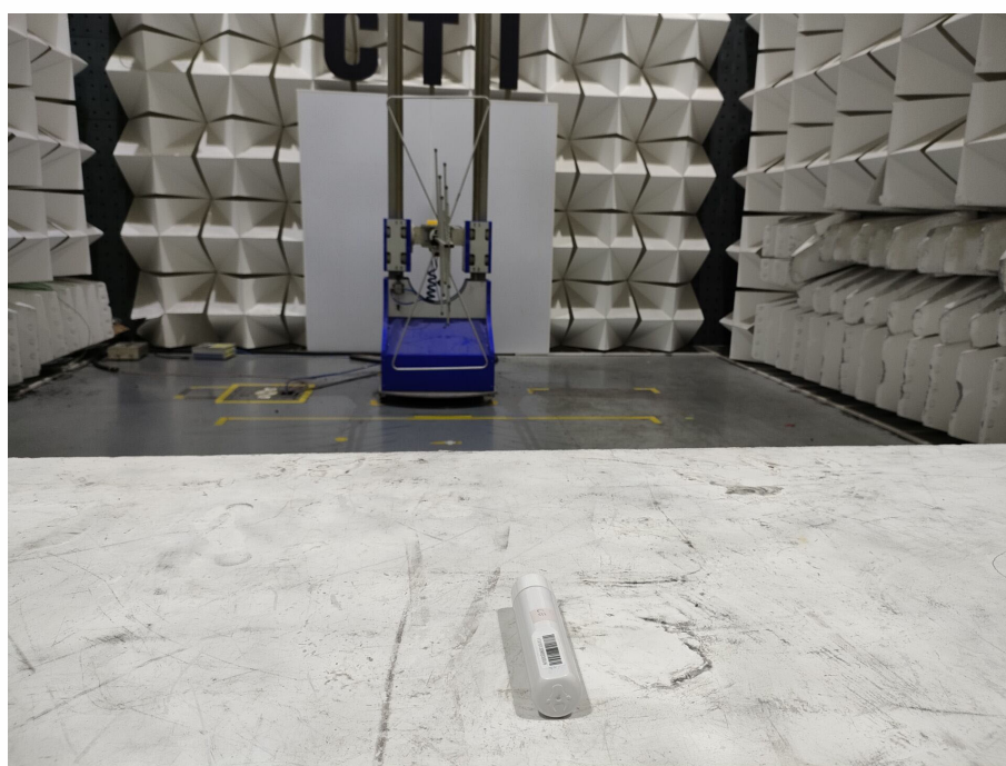
Radiated spurious emission Test Setup-4(Below 1GHz) (big) Close up
