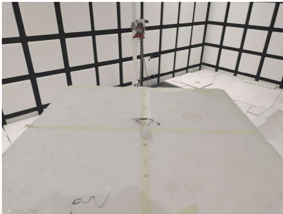
Radiated spurious emission Test Setup-3(Above 1GHz)
