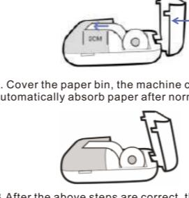
2. Cover the paper bin, the machine can automatically absorb paper after normal use.
