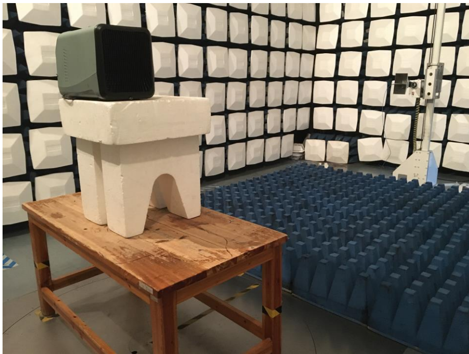
Test Setup For Radiated Emission (Above 1GHz)
