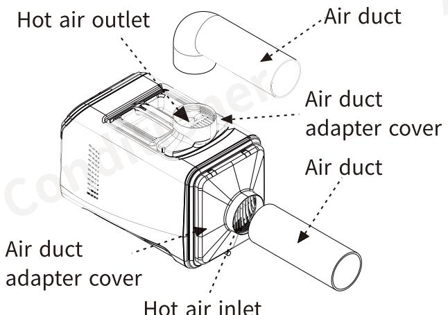
3. Install air duct if the air conditioner is used in an enclosed space:
