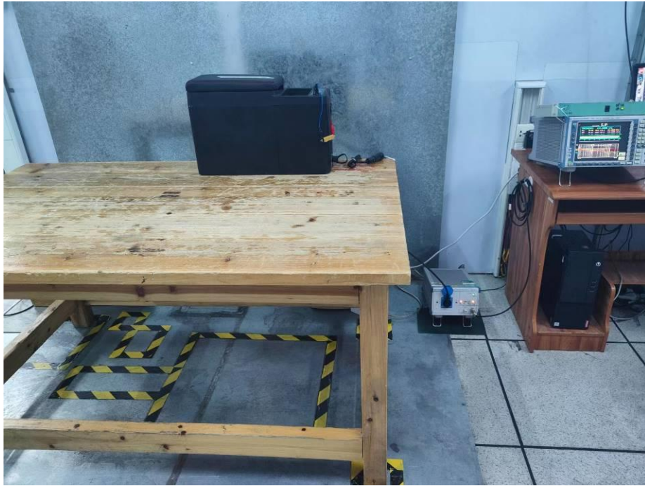
Test Setup For Conducted Emission
