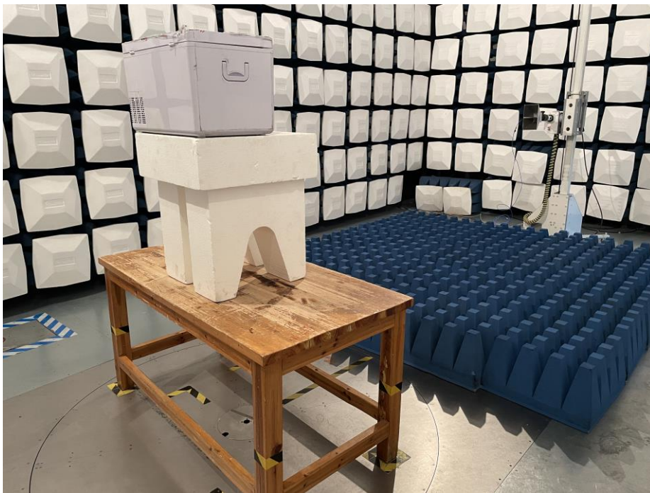
Test Setup For Radiated Emission (Above 1GHz)
