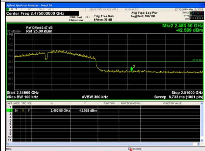
Out Of Band Emission IEEE 802.11n_Channel 9_40MHz_Antenna 0
