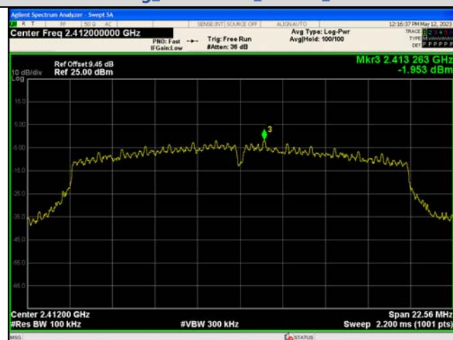
In-Band Reference Level IEEE 802.11n_Channel 1_20MHz_Antenna 0
