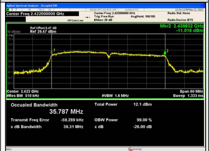
IEEE 802.11n_Channel 3_40MHz_Antenna 0
