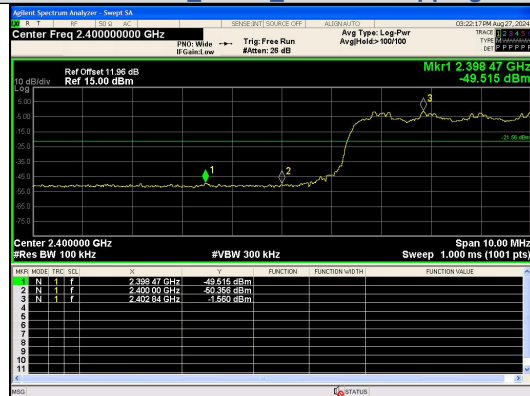
Out Of Band Emission(Left) \pi/4 DQPSK_2-DH5_Channel Hopping
