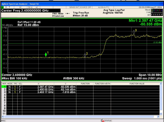
Out Of Band Emission(Left) 8DPSK_3-DH5_Channel Hopping
